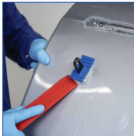
Easily remove plastic tabs after pulling is complete.
