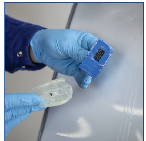
Plastic tabs are reusable and ready to pull dent after dent.
