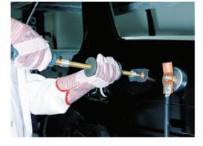
Quickest dent pulling system ever! Just weld the Spot Hammer directly on the dent and hammer away pulling the dent. Simply twist to release (magnetic ground plate optional).
