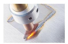
Ideal for rust repair and patching, stitch welding works by delivering an intermittent or pulsating current while rolling the tip on the sheet metal edge.
