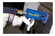
Position the weld tip on the bottom of the dent, weld, then squeeze the handle of the Pro Pull to initialize the pulling action.
