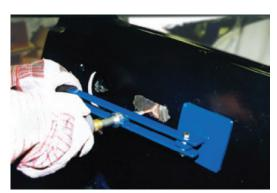
Simply weld on the shaft to the dent and use the Lever Bar to pull and straighten out dents.
